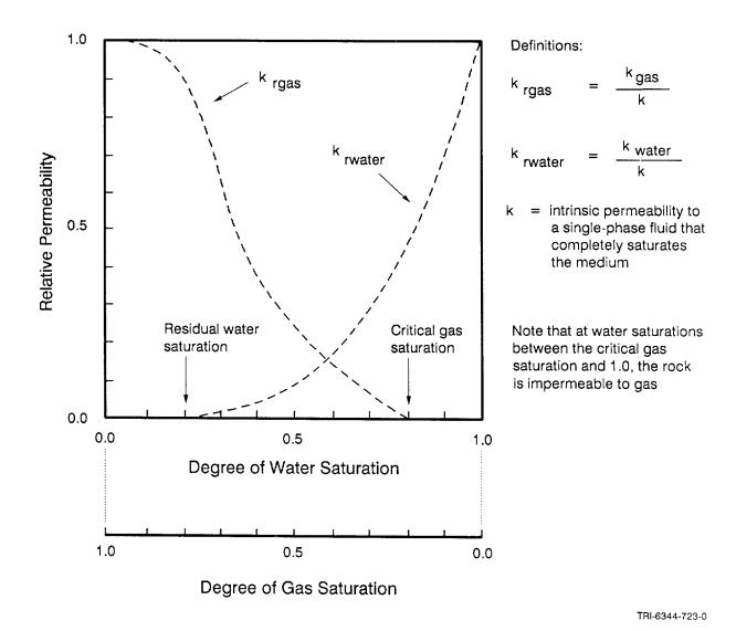
Figure 1. Definition of relative permeability to water (brine) and gas as a function of the degree of water (or gas) saturation. Also note definitions of residual water saturation and critical gas saturation.
