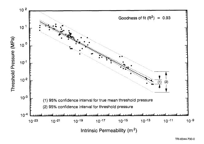
Figure 8. Plot of correlation of threshold pressure with intrinsic permeability for a composite of data from all consolidated rock lithologies. Data are from Ibrahim et al., 1970; Rose and Bruce, 1949; Thomas et al., 1968; and Wyllie and Rose, 1950.
