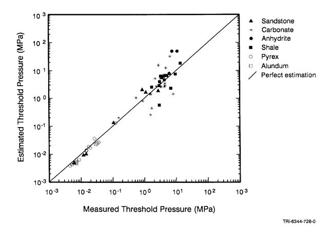
Figure 6. Plot of estimated versus measured threshold pressure for estimates based on the capillary tube model. Data are from Thomas et al. (1968), Wyllie and Rose (1950), and Ibrahim et al. (1970).
