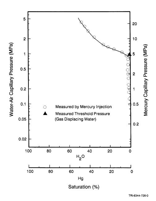
Figure 4. Plot showing an example of threshold pressure measurement by mercury injection for a 1 microdarcy (10<sup>-18</sup> m<sup>2</sup>) sandstone. (Figure adapted from Thomas et al., 1968, Figure 6.)
