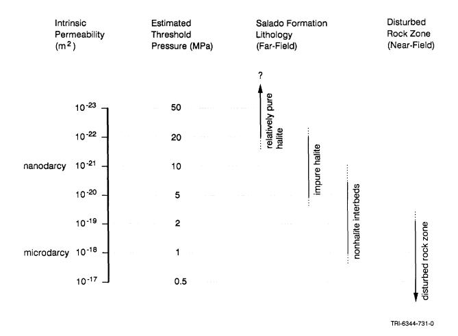
Figure 9. Plot summarizing estimated threshold pressure for various lithologic units in the Salado Formation based on correlation with intrinsic permeability.
